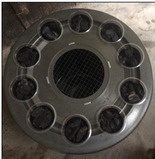
Fig. 3. Modified bucket cover for budikdamber
