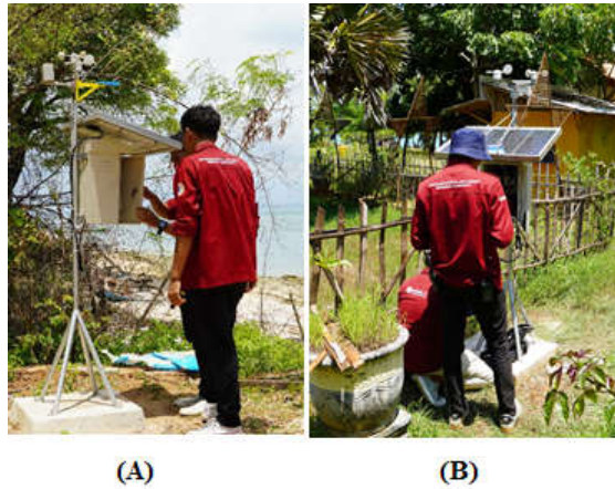
Fig. 4. AirFeel device version 3 with oxygen sensor customization, (a) device 5 was installed in the east side of the island, Ropet Beach, (b) device 7 was installed in the west side of the island, Samirun Beach.
