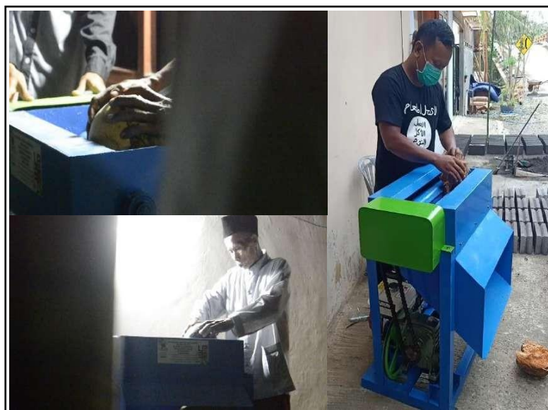
Fig. 3. Coconut Coir peeling Process using Coconut Coir peeling Machine
